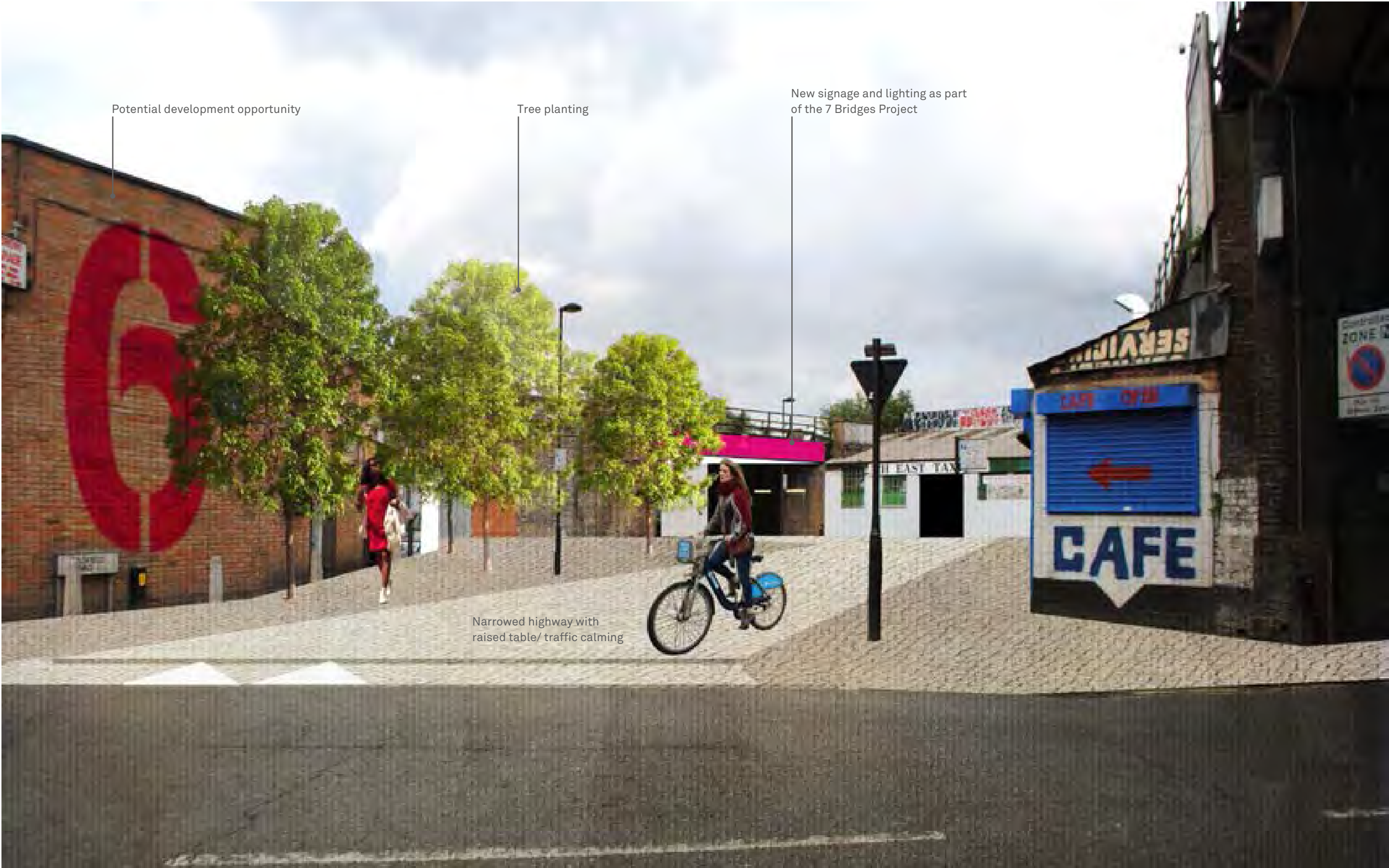
View towards Padfield Road from Herne Hil Road showing highways improvements (road narrowing, raised table) and public realm enhancements
