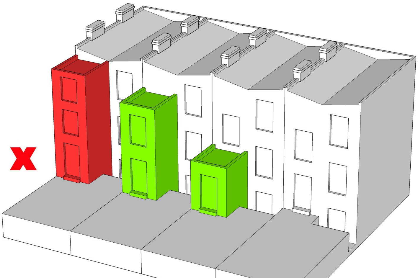
Fig 3. The closet return on the left (red) is not acceptable because it does not terminate half a storey below eaves level.
