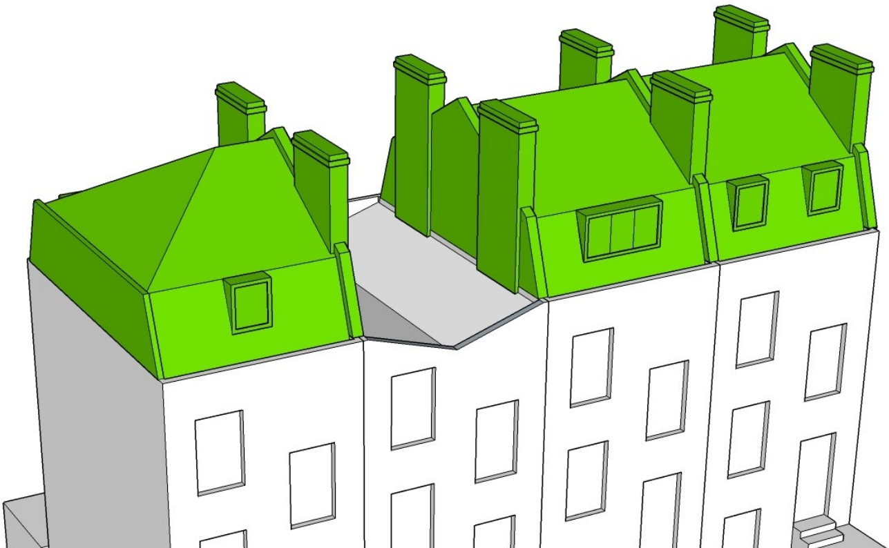
Fig. 12 This shows a rear view of the traditional mansard roof additions to a terrace of houses with London roofs which are not heritage assets. The view is of the rear shows three options for dormers - a single small dormer, a pair of dormers or a box dormer no wider than the windows below.
