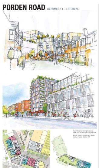
The design for Porden Road re-envisions the London terraced street. 2 storey houses face the street with dual aspect apartments above. Green planted terraces provide amenity space above the three parts of the building. The building rises from 4 storeys to echo the existing terrace at the north of the site, to 6 and then to 9 storeys on the Brixton Hill edge.
