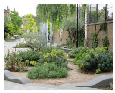
Van Gogh Walk in Stockwell was previously dominated by parking bays for local buses. In 2013-14 Transport for London and Lambeth Council installed a network of seating, new landscaped beds and planted areas. Porous bonded gravel and extensive areas of planted bedding increased the water retention capacity of this area.
