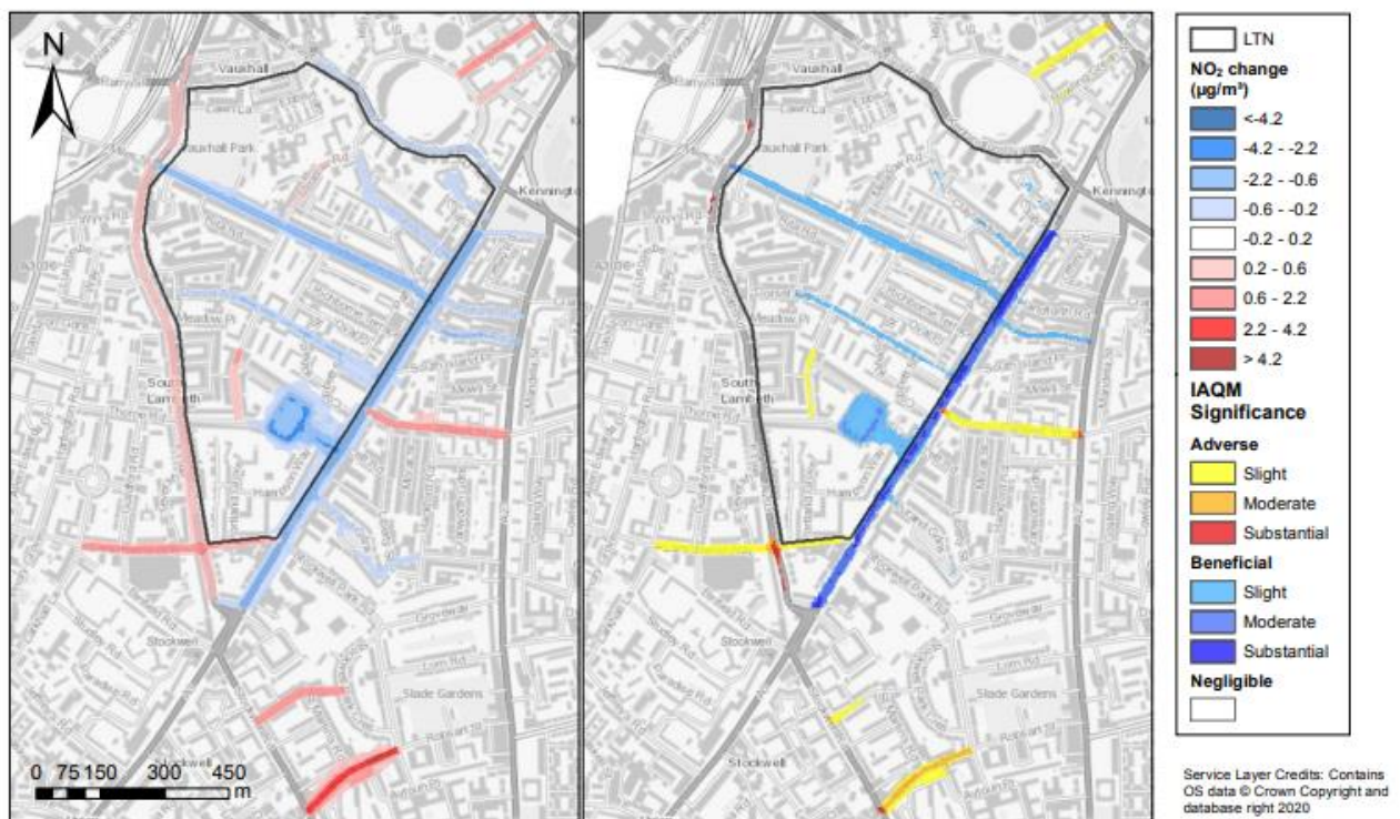
Figure 6.12: Difference plot (post-scheme minus pre-scheme) of annual average NO 2 concentrations coloured by EPUK IAQM concentration change bands (left) and EPUK IAQM impact descriptor plot coloured by EPUK IAQM significance criteria (right), Oval LTN
