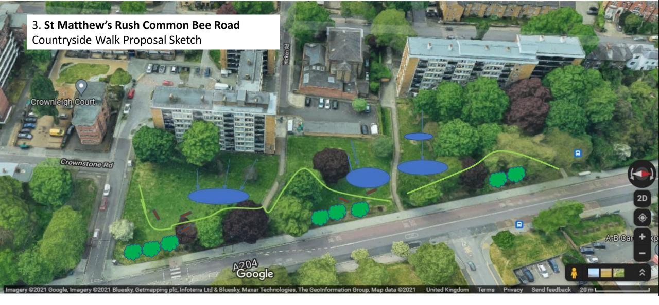
A series of rainwater ponds, holding rainwater channelled from the two blocks and low garages between. The lowest pond area will be designed to hold rainwater for longer as habitat for wildlife. The other ponds will be temporary and will overflow into this one, with meadow wildflower planting at other times. Small evergreen trees along the roadside will help to make this an attractive walk-through into Brixton with benches alongside.
