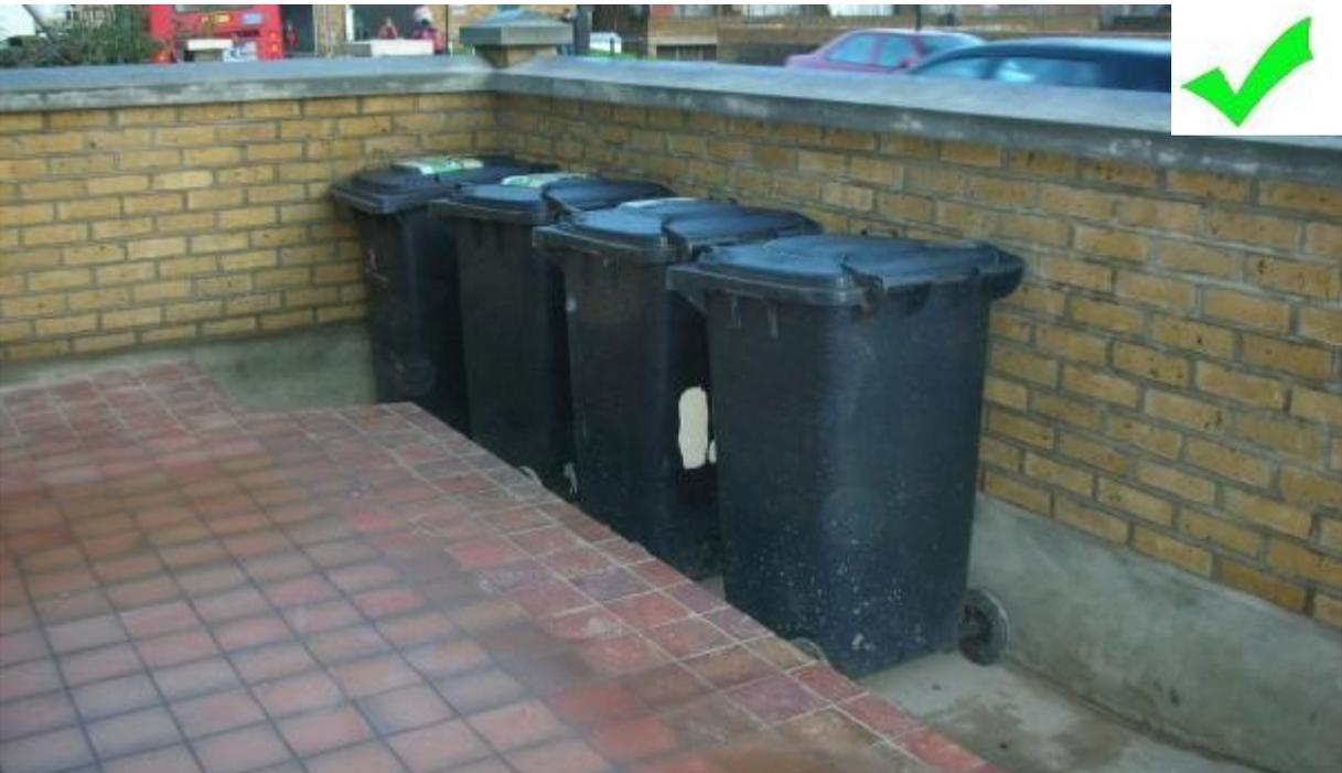
3. Part of this garden has been excavated to keep the bins out of sight from the street. Their in-ground placement allows easier access to the lids for users. The bins are wheeled up a gentle ramp for collection.
