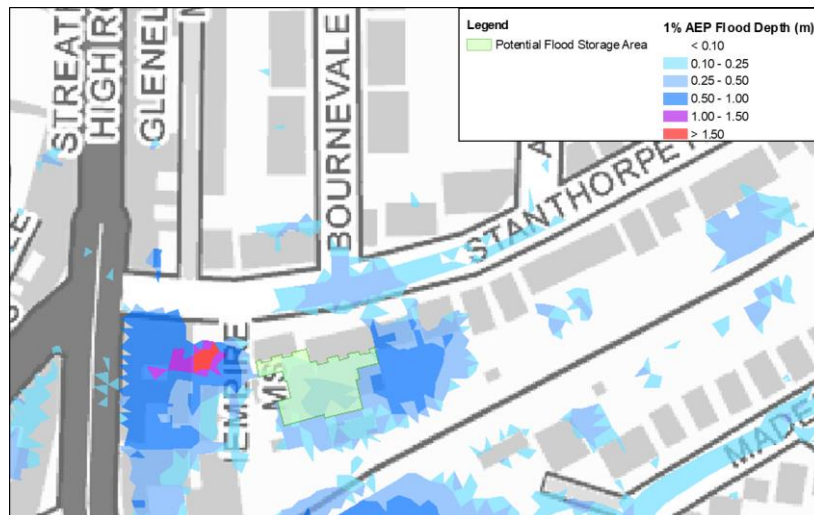
Figure 55 Proposed flood storage area and raingarden conversion within the Stanthorpe Close Estate
