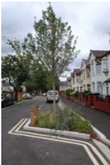
Figure 42 Example of SuDS incorporated in traffic calming measures and extended pavements (Source: SusDrain 29 )
