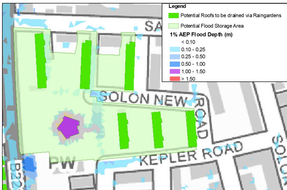
Figure 44 Indicative areas for flood storage and roof disconnections around the Solon Estate
