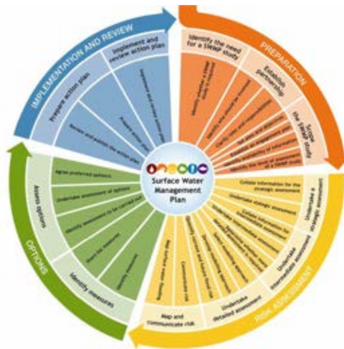
Figure 1 Wheel diagram illustrating the SWMP framework (Source: Surface Water Management Plan Technical Guidance, March 2010, DEFRA)
