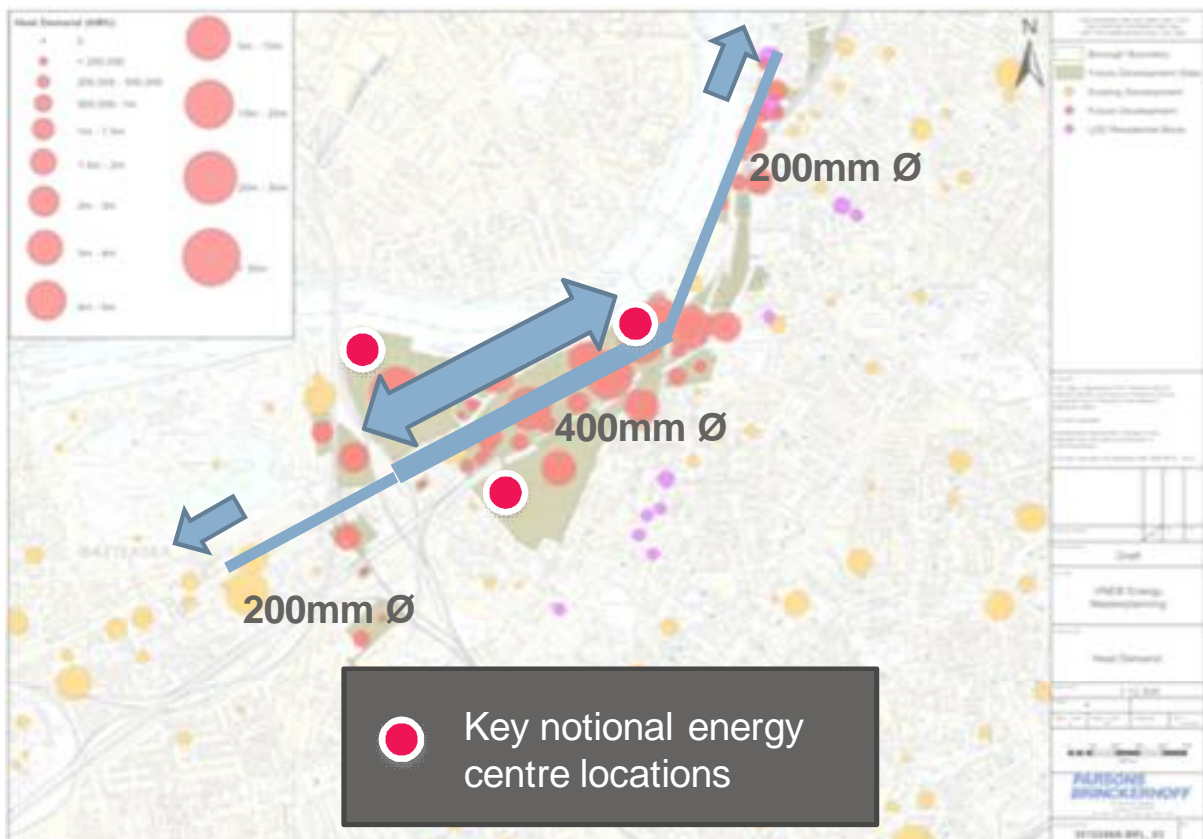
Figure 7-1 Main spine sizing illustration
