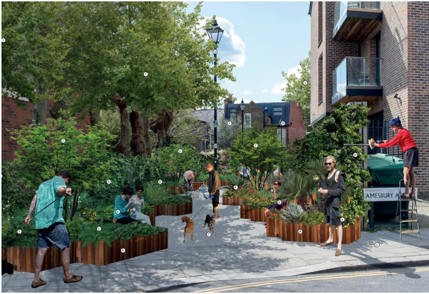
1 - Proposed small multistem trees, 3 - Existing pavement surface, 4 - Proposed sun loving exotic species, 5 - Proposed 6 - Integrated seating area, 7 - New textural surface (permeable resin bound gravel, compacted self-binding enrich sheet plus, 9 - A mixture of climbing species, 10 - Existing lamp posts to be retained.
