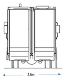
Note: any part of a building through which a waste collection vehicle passes must have a minimum clear height of 4.5m, to allow for overhead fixtures and fittings
