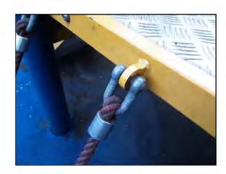
Finding: The bushes are worn or missing Action: Replace worn or missing bushes
