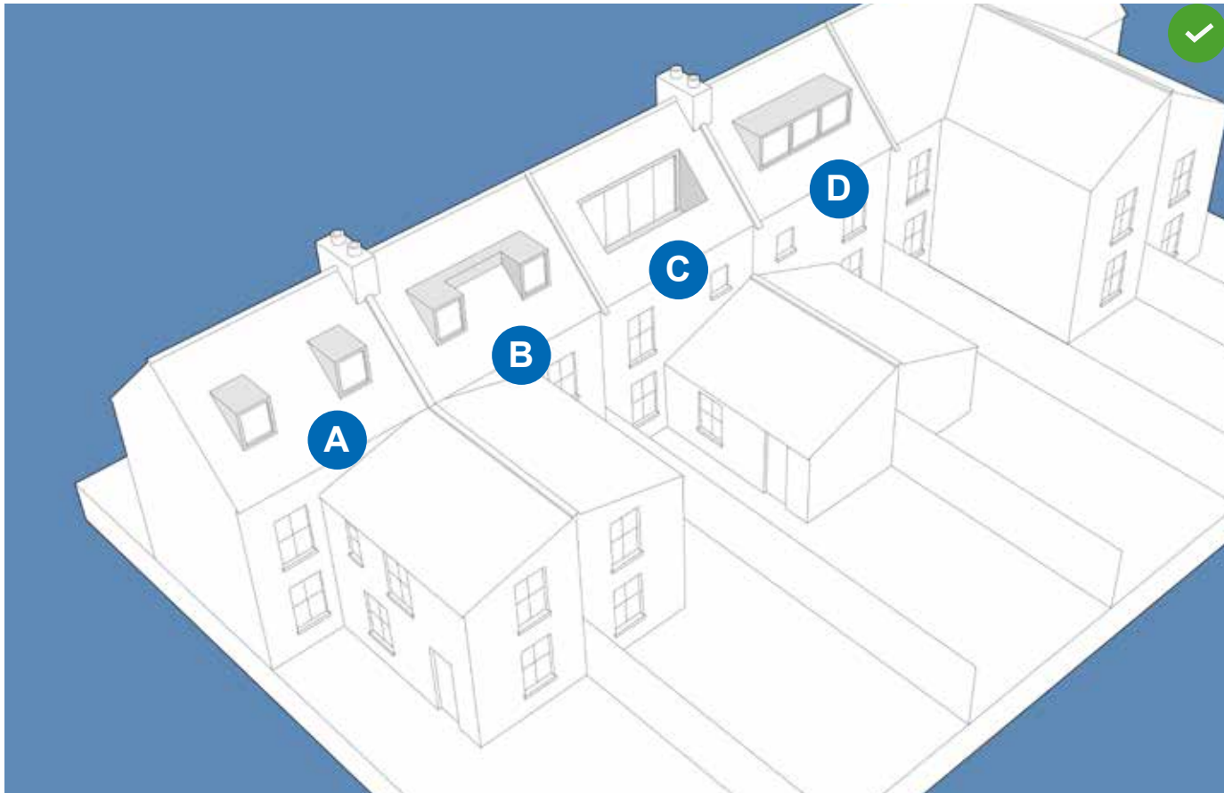
Figure 11: Acceptable rear dormers
