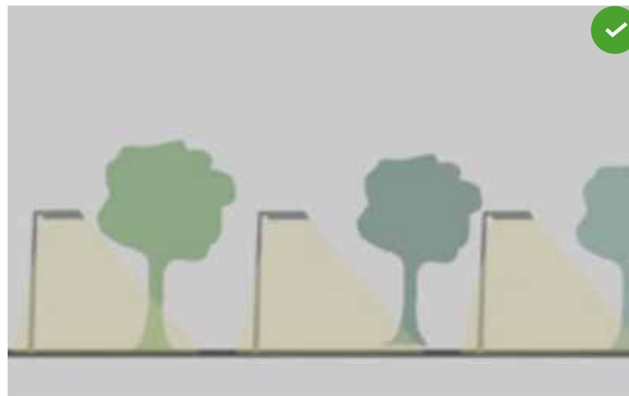
Combine shielded luminaires with short poles to minimise negative impacts of light trespass
