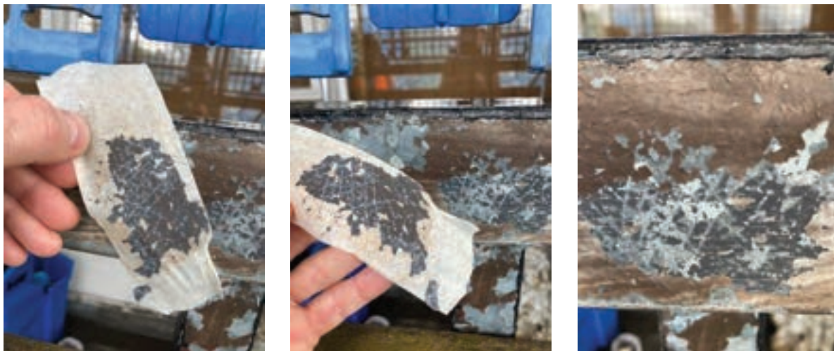
Fig 2 – Adhesion tests reveals total loss of adhesion back to the substrate.
