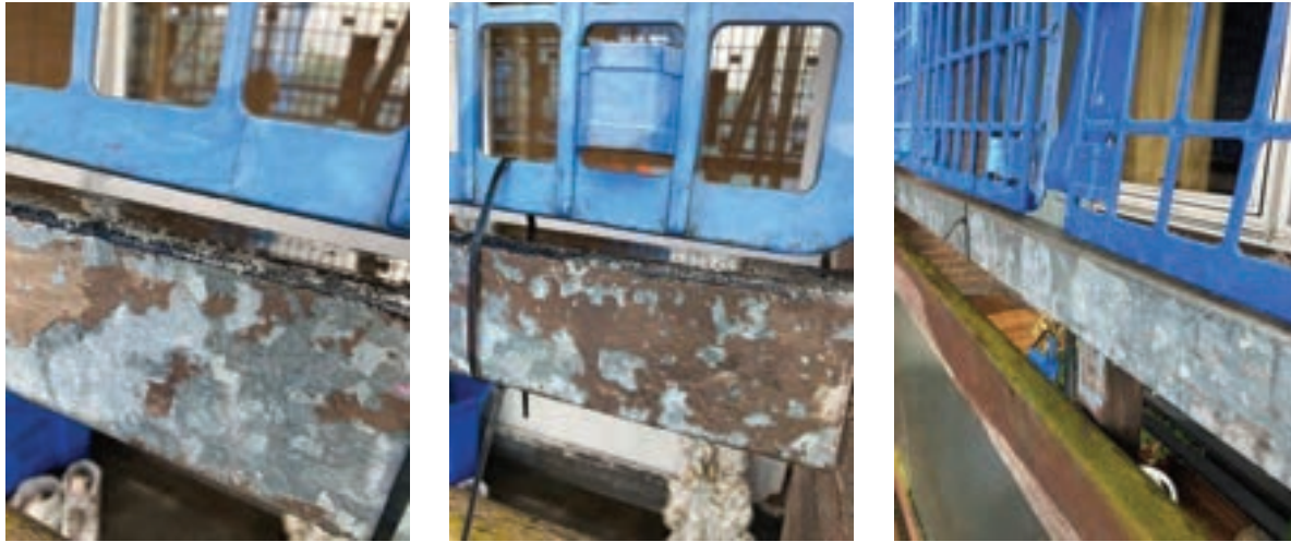
Fig 2 – Adhesion tests reveals total loss of adhesion back to the substrate.
