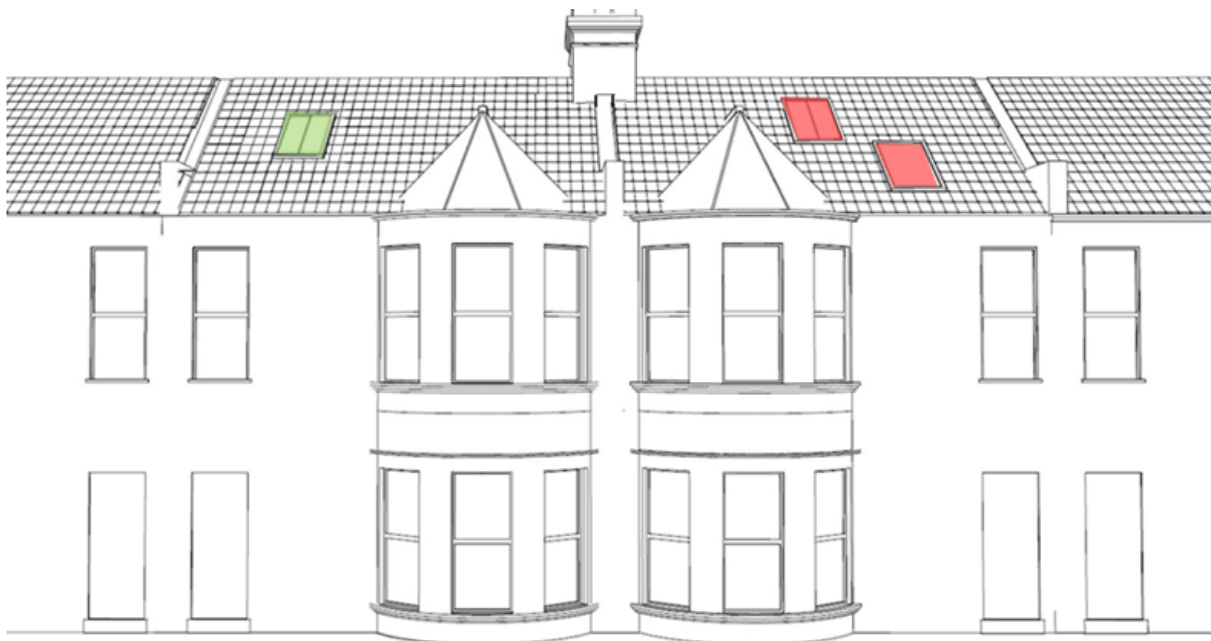
Figure 14 - The left rooflight (in green) will be supported. The right roof light locations (in red) will not be supported.
