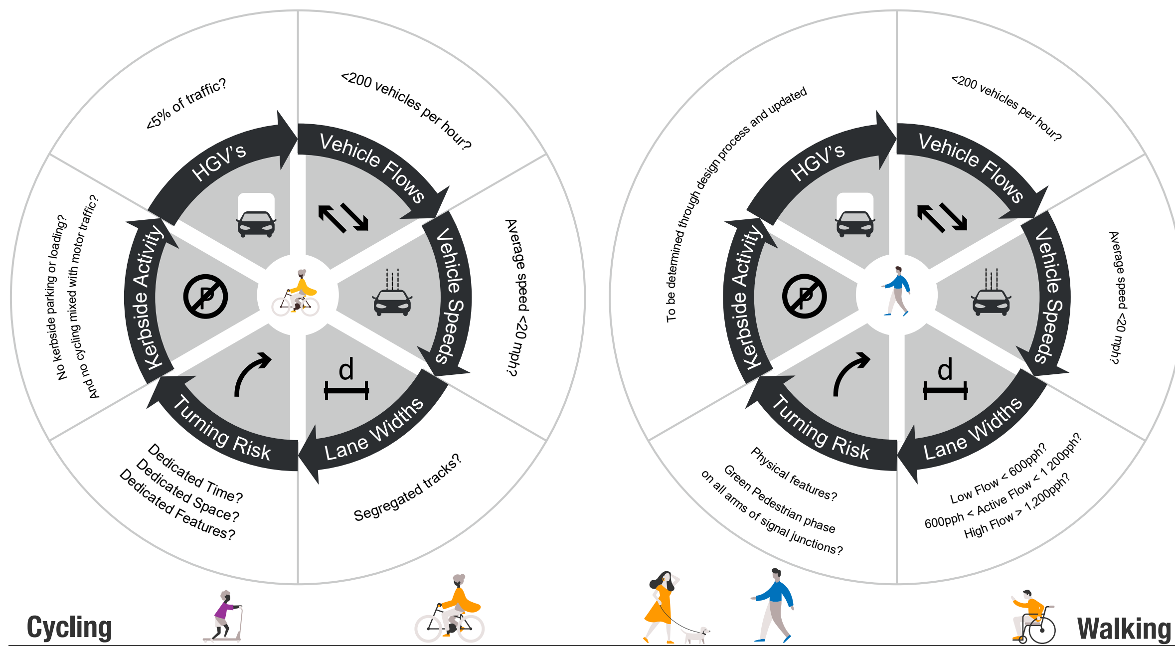
Healthy Route Criteria for walking and cycling as defined in Lambeth's 2019 Transport Strategy
