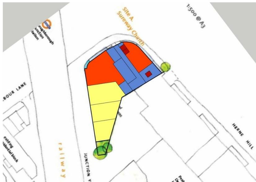
Figure 10 - Indicative Approach – Ground floor footprint. Blue is cores serving the upper floors. Red is retail, and yellow is workspace.
