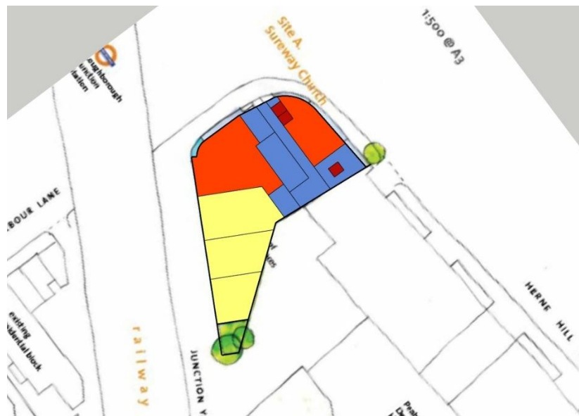
Figure 10 - Indicative Approach – Ground floor footprint. Blue is circulation serving the upper floors (lifts in crimson). Red is retail, and yellow is workspace.
