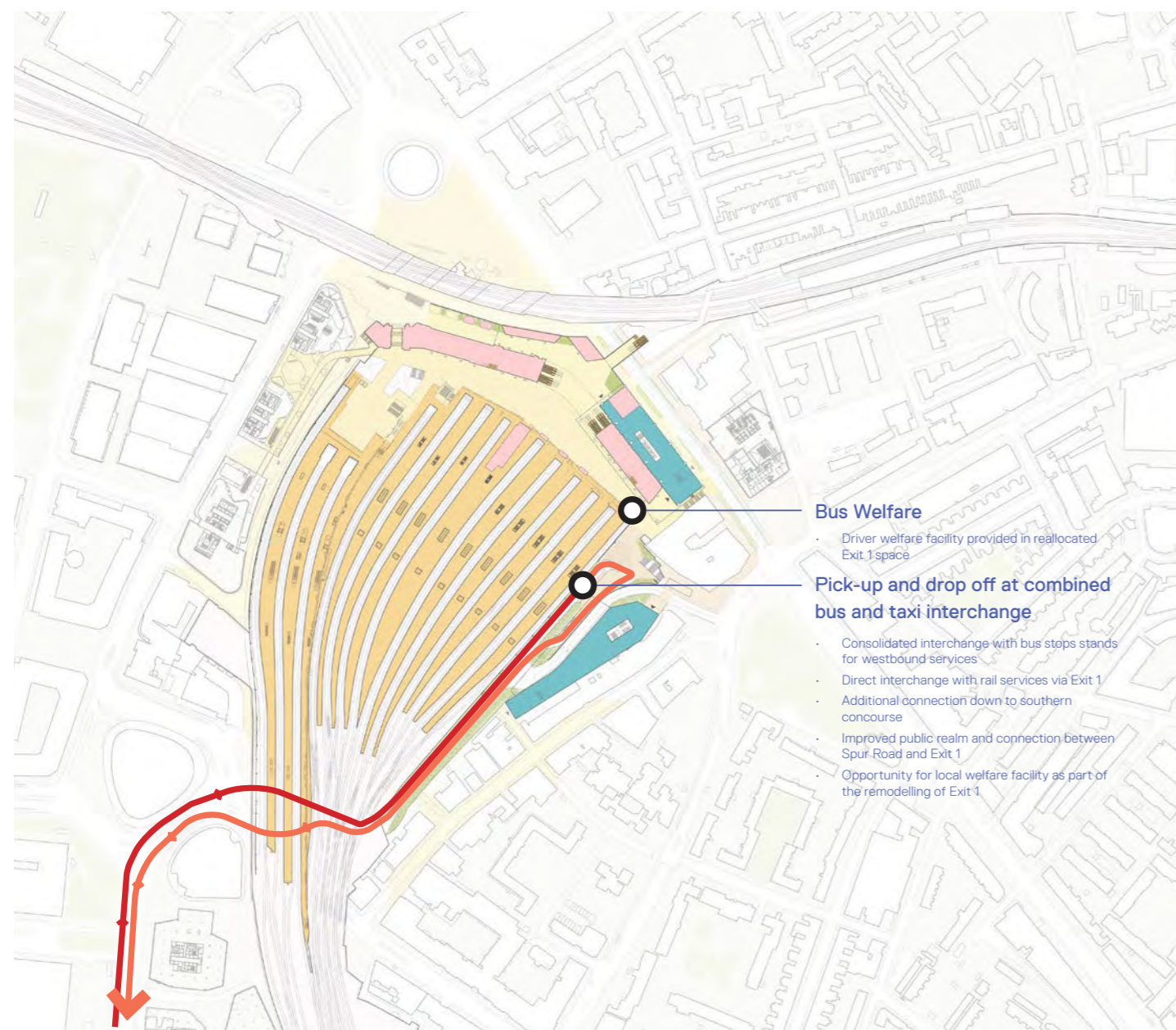
Figure 4.6: Principles of re-routing westbound services into combined bus and taxi interchange to facilitate pedestrianisation of Cab Road
