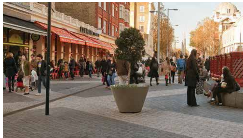
Exhibition Road outside South Kensington tube station showing improvements which features a kerb-free surface, with tactile materials to distinguish boundaries between areas for pedestrians and vehicles, plus removing street clutter. Improvements also included removing the gyratory system around South Kensington station and reducing speed limits to 20mph.
