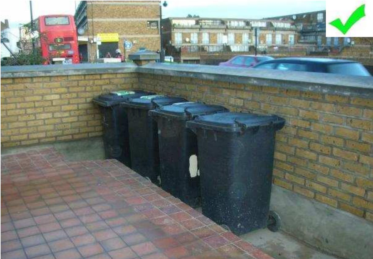
Part of this front garden has been excavated to keep the bins out of sight from the street. Their in-ground placement allows easy access to the lids. The bins are wheeled up a gentle 4
